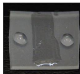
Fig. 1 Modified silicone rubber sheet wetted with water.
