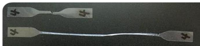
Figure 2 Shapes of test piece after elongation measurements
