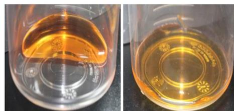
Fig.2 Water-wettability of unmodified (left) and modified (right) PMP resin vessels.
